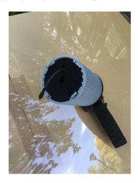
(IMPORTANT: PULL GENTLY OUT THE CABLE ALLOWING TO MOUNT MICROPHONE AS NEXT STEP WITH A GENEROUS CABLE U-BEND)
