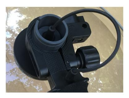
STEP 3. SECURE THE HANDLE CYLINDER "STOPPER" ATTACHED TO CABLE INSIDE THE TUBE WITH THE CABLE GROMMIT ALIGNED BACK OF TUBE \*PLACED AS PHOTO TIP! LOOSEN UP THE KNOB, PLACE CYLINDER INSIDE, THEN SECURE KNOB AGAIN.
