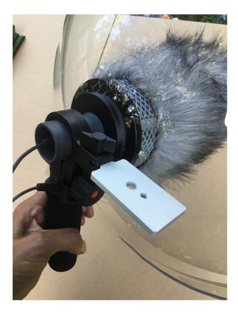
(**PHOTO:** LOOSEN UP THE TOP SCREW OF THE **HANDLE**, SLIDE IN THE **TRIPOD MOUNT** AND THE SECURE AGAIN THE TOP SCREW)
