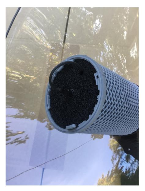
IMPORTANT: MIC IN FOCUS ONLY WHEN THE BACK OF THE MIC BODY IS ALIGNED WITH THE FOAM AS PHOTO ABOVE. PLEASE ALLOW THE CABLE TO FORM A U-SHAPE.
