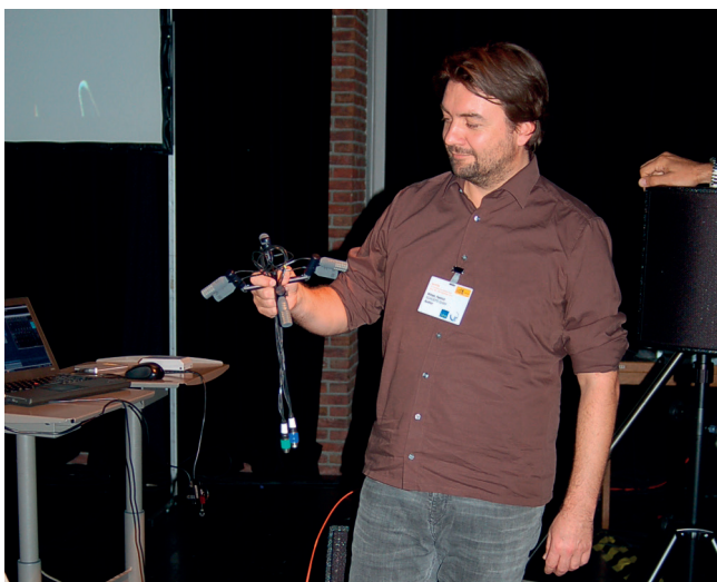
Fig. 4: A prototype of the ORTF-3D system at the ICSA conference in 2015. Eight supercardioids, horizontal distance 20 cm, vertical distance 0, angle 90°.
