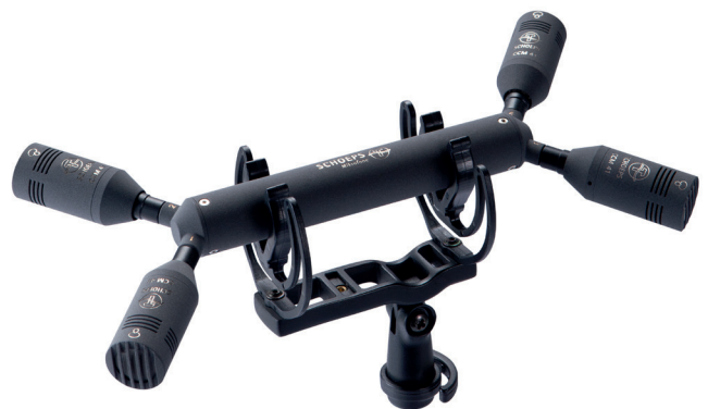
Fig. 3: Four-channel "ORTF Surround" system; four supercardioids, 10 / 20 cm spacing, 80° / 100° angles.
