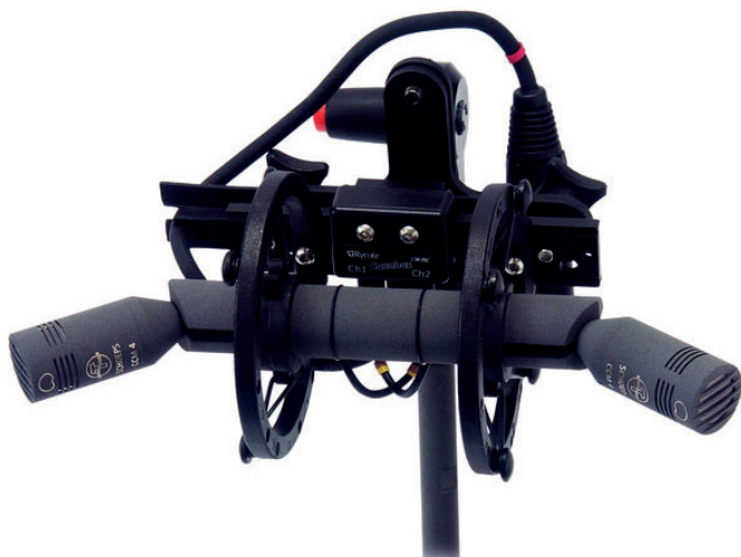
Fig. 2: Two-channel ORTF system in a suspension designed for use within a windscreen; two cardioids, 17 cm, 110°.
