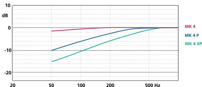
Low-frequency response curves of the two capsule types (P and XP) compared to the standart MK 4 (measured at a 60 cm equivalent distance).
