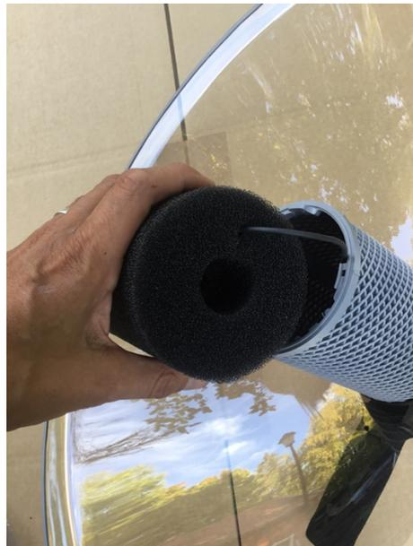
(**IMPORTANT:** USE BOTH HANDS AND GENTLY SLIDE THE CABLE THRU THE SMALLER HOLE OF THE FOAM UNTIL VISIBLE AT THE OTHER END OF THE HOLDER, (FRONT) WHERE THE MICROPHONE WILL BE MOUNTED)
