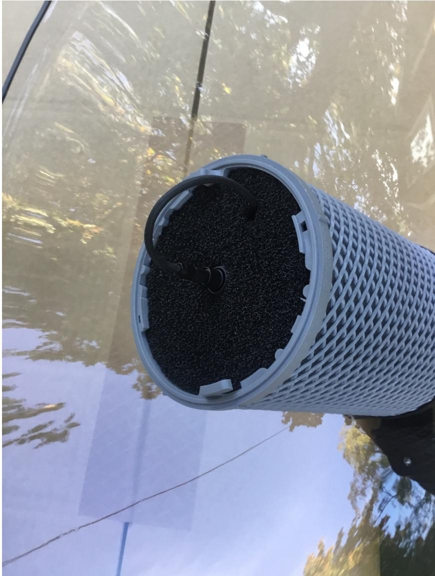
**IMPORTANT: MIC IN FOCUS ONLY WHEN THE BACK OF THE MIC BODY IS ALIGNED WITH THE FOAM AS PHOTO ABOVE. PLEASE ALLOW THE CABLE TO FORM A U-SHAPE.**
