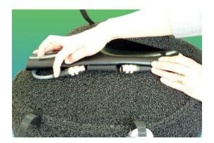
Protect the connected plugs by putting them into the sleeve (if existing)
