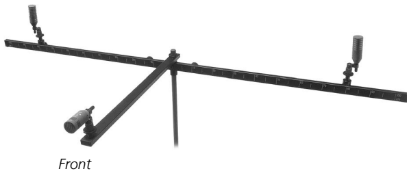
OCT 2 setup: The center-channel microphone is shifted forward
